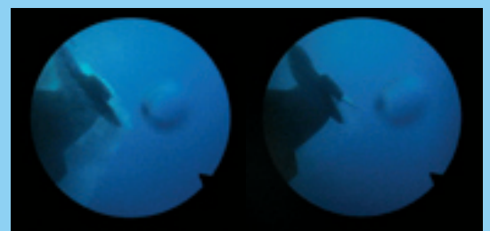
POD propeller observed through borescope, with and without cavitation (of design condition).
